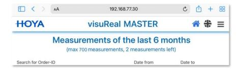
• As soon as only 25 measurements are available on the visuReal MASTER, a warning appears on the start page requesting to delete measurements. You can either ignore this request or switch to the history page to delete measurements.
